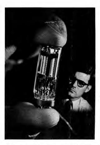
PHOTOMULTIPLIER TUBE held by Joe Vieira (8122) was holographically analyzed in the Photomechanics Lab to detect vibration problems in one of 10 dynodes (components in upper portion of tube).
